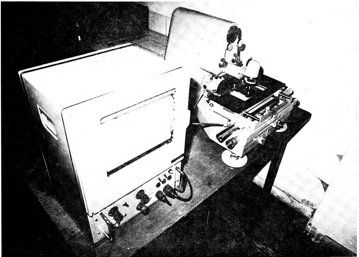
Fig. 4. Photography of the recording microphotometer used for measurements of the modulation transfer function of photographic materials
