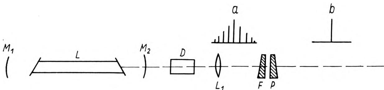
Fig. 2. Filtering of the beam by means of an external element
