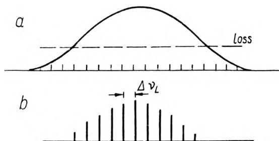
Fig. 1. The course of a laser gain and longitudinal modes:  $a$  — gain curve,  $b$  — laser output
