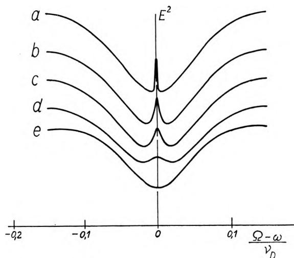
Fig. 5. Gain curves of the gas laser with the intracavity absorber for the varying Lorentz width of the absorber
