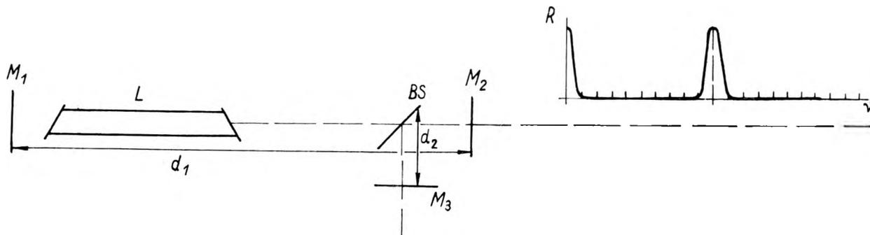
Fig. 3. Scheme of Fox-Smith interferometer
