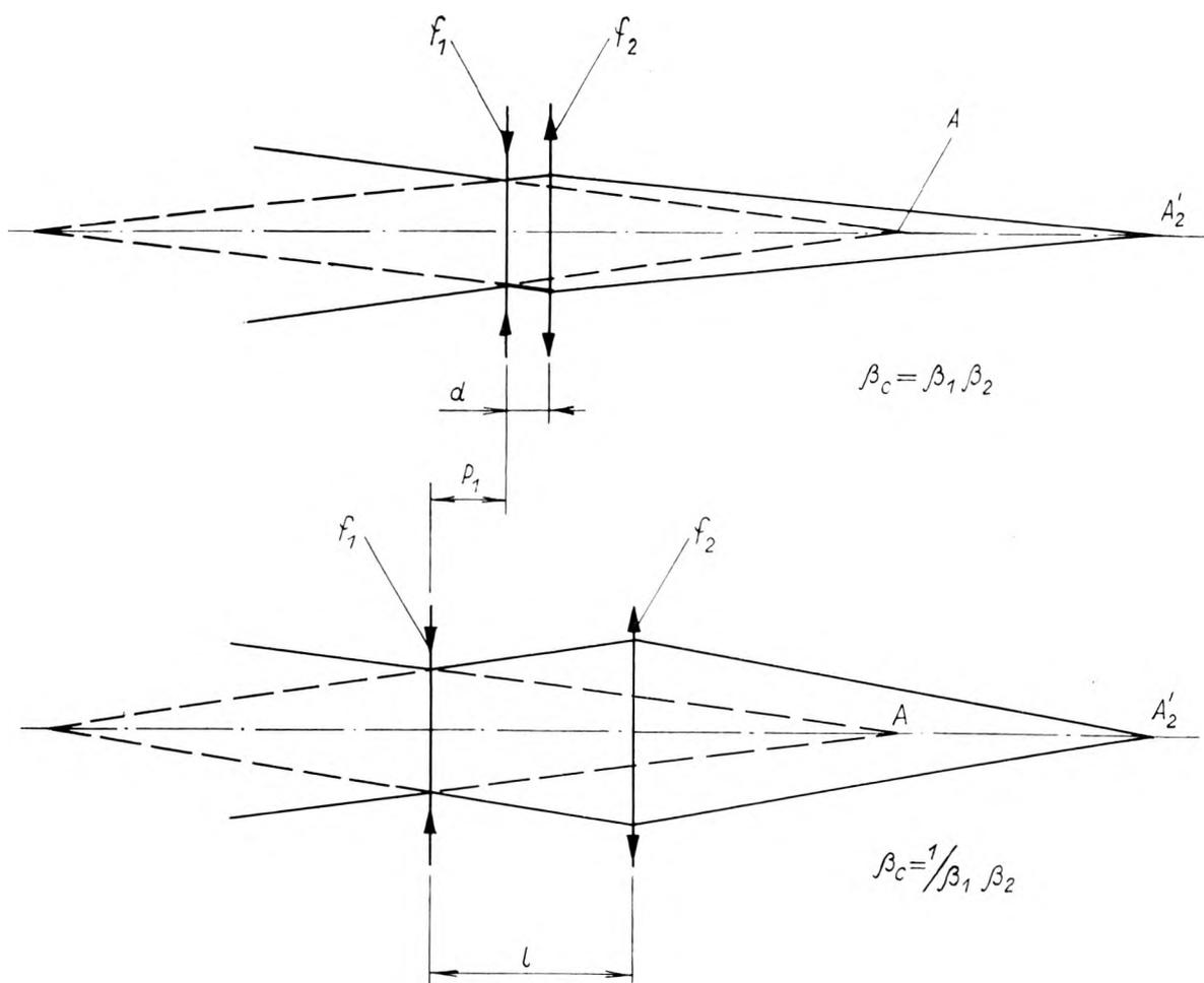
Fig. 1. An ideological scheme of a two-component solution for a pancratic optical system producing a direct image, supplied with the linear movement of elements
