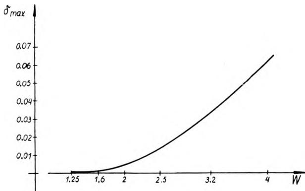
Fig. 3. Dependence between the extremal value of the image position deviation and the total magnification variation factor for the two-component pancratic optical system
