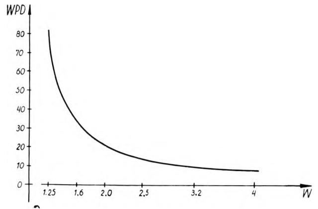
Fig. 4. Graph of the deviation improvement factor for the two-lens pancratic systems
