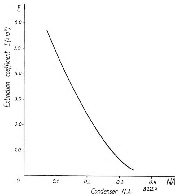
Fig. 2. A decrement of the instrumental extinction  $E$  of the system as a function of the condenser aperture  $NA$
