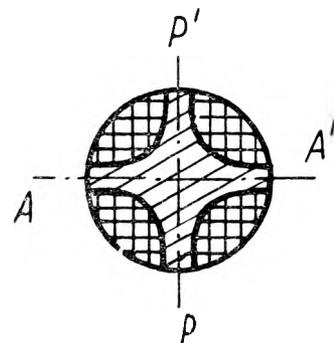
Fig. 5. An image of the exit pupil of the polarization microscope objective with crossed analyzer and polarizer
