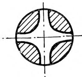
Fig. 4. Aperture diaphragm under the condenser. A view from the upper side
