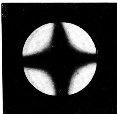
Fig. 1. "Conoscopiccross" in the exit pupil of the objective in the polarization objective for crossed polarizer and analyzer. Objective aperture 0.40
