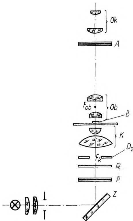
Fig. 3. Scheme of the polarization microscope with the special aperture diaphragm  $D_2$  placed in the focal plane of the condenser
