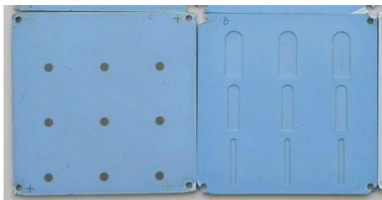
Fig. 5. Two exemplary laminates before cutting into single structures
