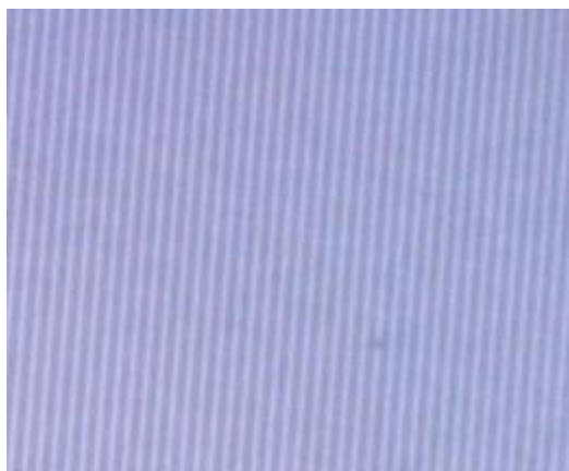
Fig. 4. The result of the single photoresist exposure. 89 pulses, Pulse Repetition Rate PRF = 10 Hz
