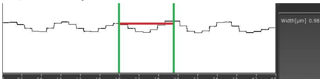
Fig. 6. Profile measurement of the distance between interference fringes
