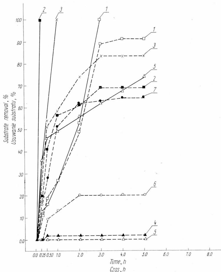
Fig. 3. Biodegradation dynamics of preaerated phenolic substrates in activated sludge process. For the legend see Fig. 1
