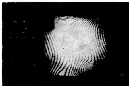
Fig. 7. Holographic interferograms obtained during wavefront reconstruction from the double-exposure holograms: p_1 = 25.0 at, p_2 = 30.0 at
