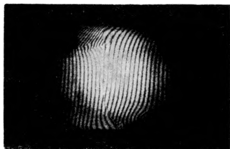
Fig. 2. Holographic interferograms obtained during wavefront reconstruction from the double-exposure holograms: p_1 = 5.0 at, p_2 = 10.0 at
