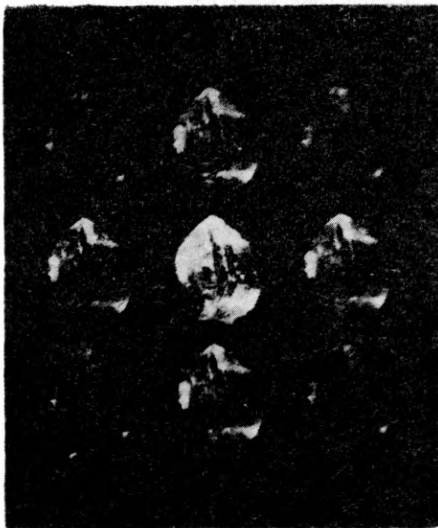
Fig. 7. Multiple images of a 3-D object. Dimensions of the sampling filter were matched according to the eq. (15)
