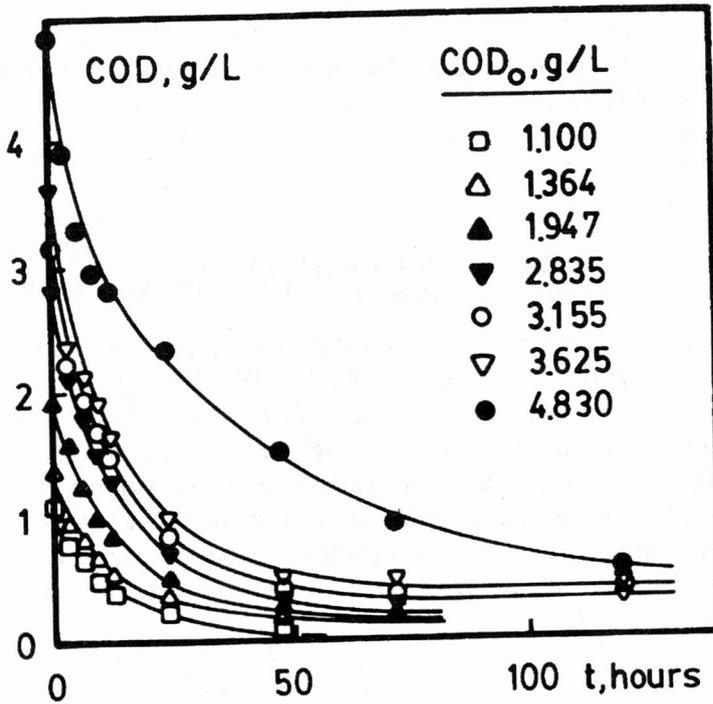
Fig. 1. Evolution of COD degraded with digestion time
