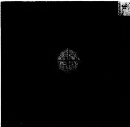
Fig. 6. Photomicrography of the diffraction pattern of the cement dust
