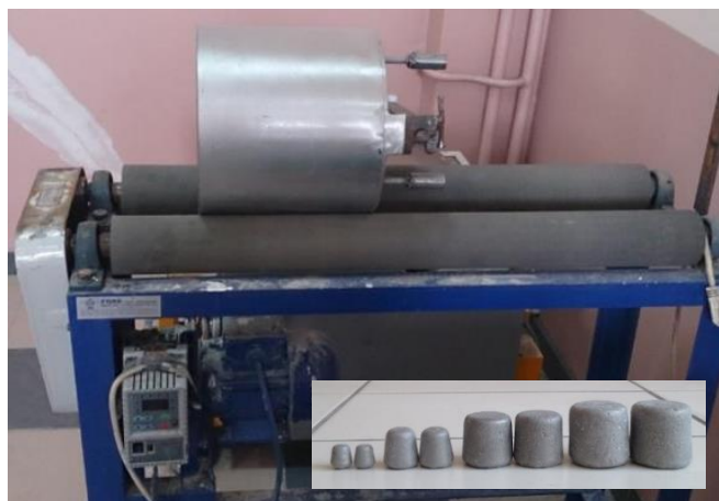
Fig. 2. Laboratory ball mill and cylpebs used in the tests
