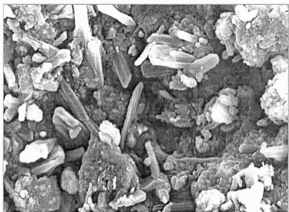
Fig. 5. SEM image of ODA-modified clinoptilolite-rich tuff; magnification 3000 \times
