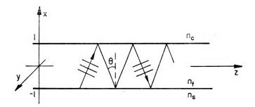
Fig. 1. An ideal dielectric slab waveguide – choice of coordinates
