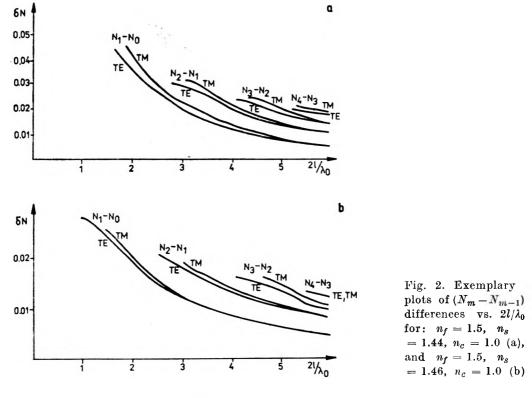
The magnitudes of limitations resulting from the second condition can be estimated from the plots of  $(N_m - N_{m-1})$  vs.  $2l/\lambda_0$  (Fig. 2). MARCUSE [18] (p. 134) derived the following approximated dependence of the difference between propagation constants of two neighbour modes on the waveguide thickness 2l
