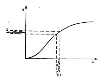
Fig. 3. The perturbed waveguide works as a modulator projecting the a(z) distribution on N(z)
