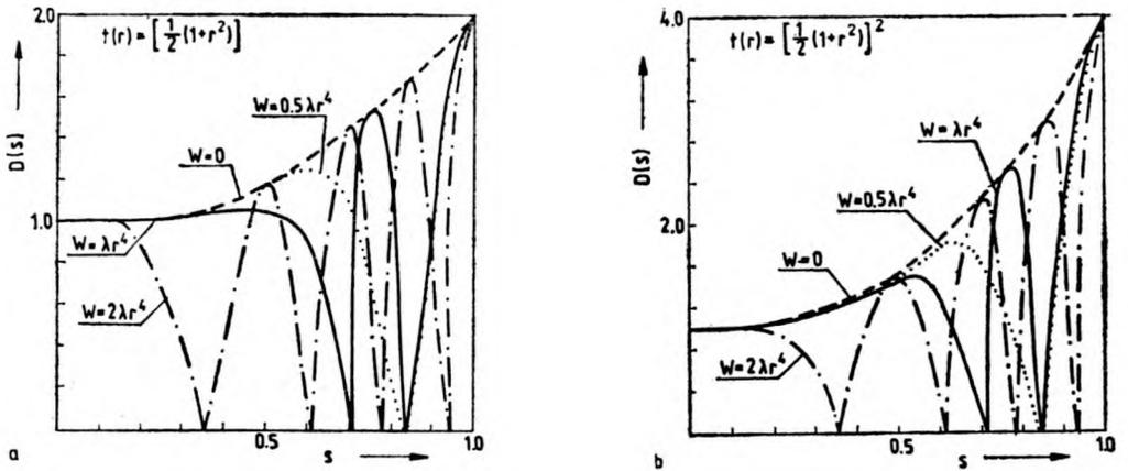
Fig. 5. Contrast change  $D(s)$  for amplitude test in the optical system with aberrations  $W(r) = 0.5\lambda r^4, \lambda r^4, 2\lambda r^4$  apodized with the function:  $t(r) = 1/2(1 + r^2)$ ,  $m = 0$  (a),  $t(r) = [1/2(1 + r^2)]^2$ ,  $m = 0$  (b)
