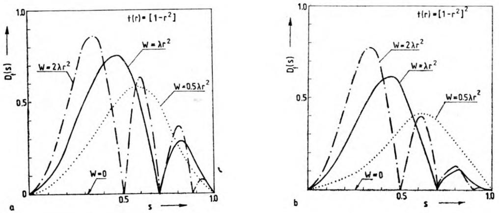
Fig. 12. Contrast change  $D(s)$  for phase test in the optical system with aberrations  $W(r) = 0.5\lambda r^2, \lambda r^2, 2\lambda r^2$  apodized with the functions:  $t(r) = 1 - r^2, m = 0$  (a),  $t(r) = (1 - r^2)^2, m = 0$  (b)
