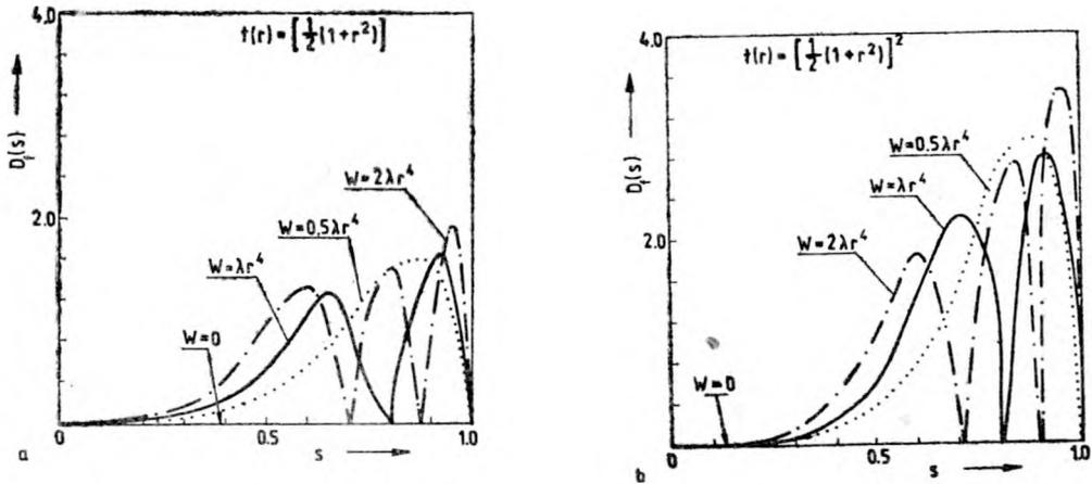
Fig. 11. Contrast change  $D(s)$  for phase test in the optical system with aberrations  $W(r) = 0.5\lambda r^4, \lambda r^4, 2\lambda r^4$  apodized with the functions  $t(r) = 1/2(1+r^2), m = 0$  (a),  $t(r) = [1/2(1+r^2)]^2, m = 0$  (b)
