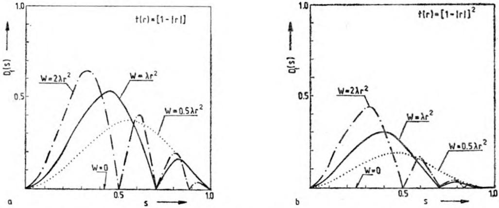
Fig. 14. Contrast change  $D(s)$  for phase test in the optical system with aberrations  $W(r) = 0.5\lambda r^2, \lambda r^2, 2\lambda r^2$  apodized with the functions:  $t(r) = 1 - |r|$ ,  $m = 0$  (a),  $t(r) = (1 - |r|)^2$ ,  $m = 0$  (b)
