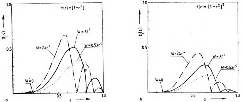
Fig. 13. Contrast change  $D(s)$  for phase test in the optical system with aberrations  $W(r) = 0.5\lambda r^4, \lambda r^4, 2\lambda r^4$  apodized with the functions:  $t(r) = 1 - r^2, m = 0$  (a),  $t(r) = (1 - r^2)^2, m = 0$  (b)
