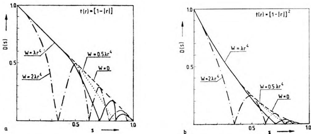
Fig. 9. Contrast change  $D(s)$  for amplitude test in the optical system with aberrations  $W(r) = 0.5\lambda r^4, \lambda r^4, 2\lambda r^4$  apodized with the functions:  $t(r) = 1 - |r|$ ,  $m = 0$  (a),  $t(r) = (1 - |r|)^2$ ,  $m = 0$  (b)
