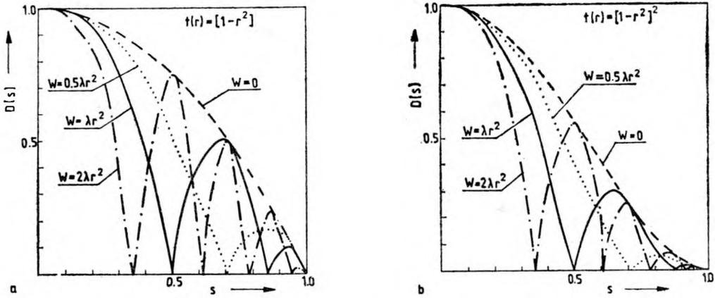
Fig. 6. Contrast change  $D(s)$  for amplitude test in the optical system with aberrations  $W(r) = 0.5\lambda r^2, \lambda r^2, 2\lambda r^2$  apodized with the functions:  $t(r) = 1 - r^2, m = 0$  (a),  $t(r) = (1 - r^2)^2, m = 0$  (b)
