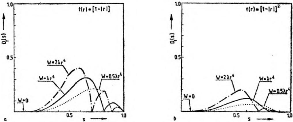
Fig. 15. Contrast change  $D^t(s)$  for phase test in the optical system with aberrations  $W(r) = 0.5\lambda r^4, \lambda r^4, 2\lambda r^4$  apodized with the functions:  $t(r) = 1 - |r|$ ,  $m = 0$  (a),  $t(r) = (1 - |r|)^2$ ,  $m = 0$  (b)
