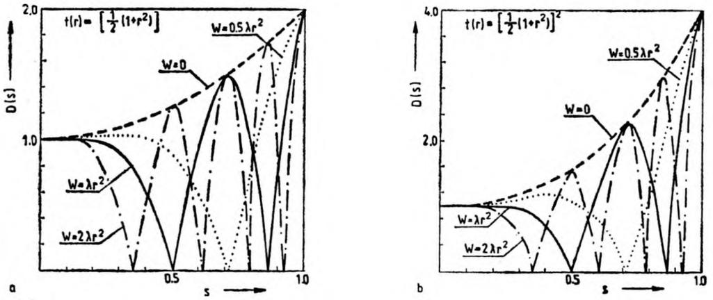
Fig. 4. Contrast change  $D(s)$  for amplitude test in the optical system with aberrations:  $W = 0.5 \lambda r^2, \lambda r^2, 2\lambda r^2$  apodized with the function  $t(r) = 1/2 (1 + r^2)$ ,  $m = 0$  (a),  $t(r) = [1/2(1 + r^2)]^2$ ,  $m = 0$  (b)
