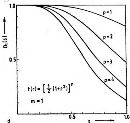
Fig. 1. The effect of amplitude apodization  $t(r)$  on the image contrast of amplitude test for:  $t(r) = 1/2(1+r^2)$  (a),  $t(r) = [1/2(1+r^2)]^2$  (b),  $t(r) = [1/2(1+r^2)]^p$ ,  $p = 1, 2, 3, 4$ ;  $m = 0$  (c),  $t(r) = [1/2(1+r^2)]^p$ ,  $p = 1, 2, 3, 4$ ;  $m = 1$  (d)
