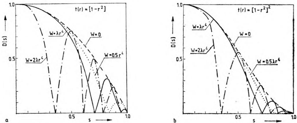
Fig. 7. Contrast change  $D(s)$  for amplitude test in the optical system with aberrations  $W(r) = 0.5\lambda r^4, \lambda r^4, 2\lambda r^4$  apodized with the functions:  $t(r) = 1 - r^2, m = 0$  (a),  $t(r) = (1 - r^2)^2, m = 0$  (b)
