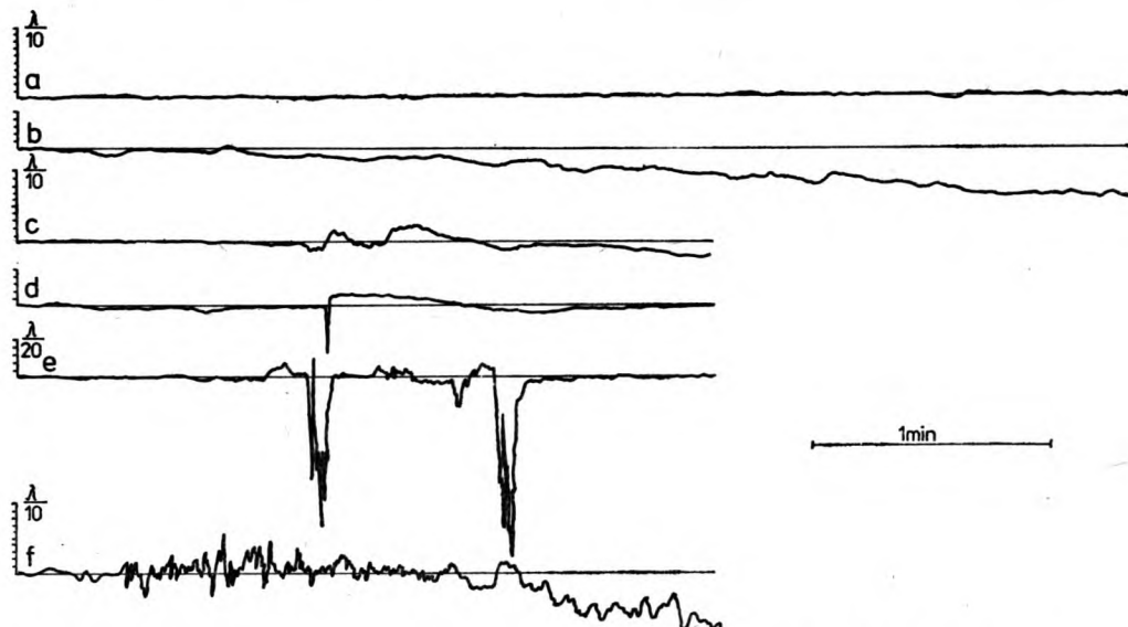
Fig. 3. Influence of the external perturbations on the random phase shifts of the interfering light beams. Assuring special stabilization conditions of the external parameters (a), typical perturbations under normal measurement conditions: effect of systematic phase change—the swimming zero (b), directing of a low flux of heated air on the measurement chamber housing (c), striking the bench plate (d), approaching the hand to the object beam (e), air rotation around the open measuring chamber (f)
