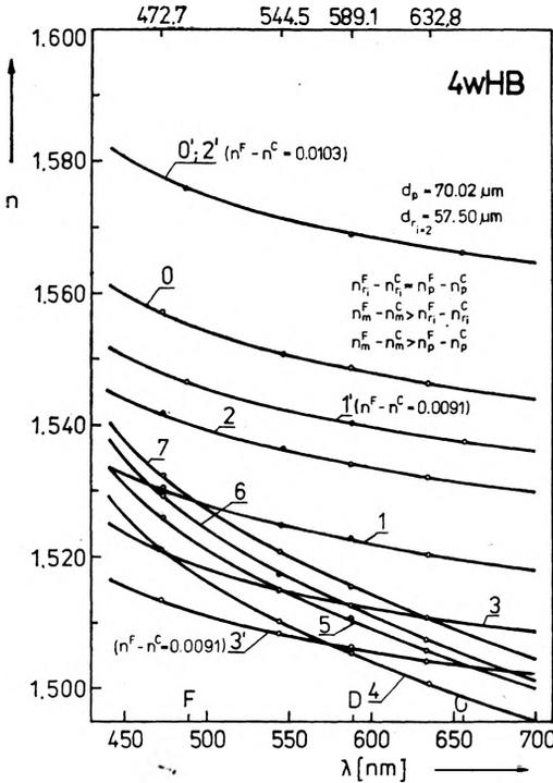
Fig. 6. Dispersion curves of fibre 4wHB (internal layers — 0, 1, and 2, cladding — 3), immersion fluids (curves 4, 5, 6 and 7) and the initial glasses used for the three internal layers and cladding (curves 0, 1', 2' and 3')
