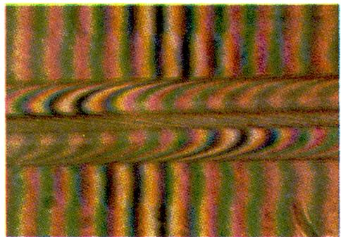
Fig. 2. Splitting of the pattern of a high-aperture optical fibre, 2wLS, in the fringe interference field: **a** – objective magnification  $10\times$ , photograph magnification  $130\times$ , **b** – objective magnification  $40\times$  ( $n_m = n_p = 1.5682$ ,  $t = 17.5^\circ\text{C}$ )
