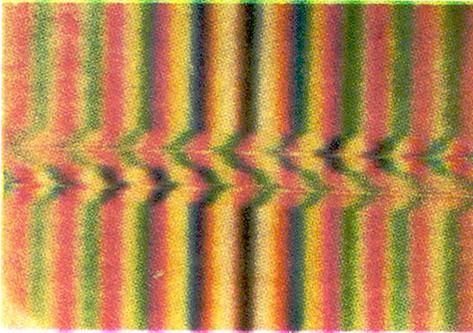
Fig. 1. Complete splitting of the pattern of a two-layer optical fibre, 2wBc, in the striated interference field:  $n_m = n_p = 1.5373$ . Photograph magnification  $130\times$ ,  $t = 19.7^\circ\text{C}$
