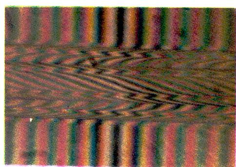
Fig. 3. Splitting of the pattern of a four-layer optical fibre, 4wHB [3], in the fringe interference field: **a** – objective magnification  $10\times$ , photograph magnification  $130\times$ , **b** – objective magnification  $20\times$ , photograph magnification  $260\times$  ( $n_m = n_p = 1.5083$ ,  $t = 17.5^\circ\text{C}$ )
