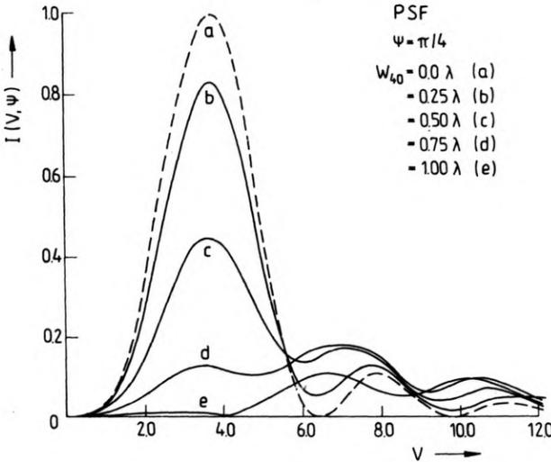
Fig. 3. Intensity point spread of polarizing microscope in the presence of third-order spherical aberration:  $\Psi = \pi/4$ ;  $W_{40} = 0.0, 0.25\lambda, 0.50\lambda, 0.75\lambda$  and  $1.0\lambda$
