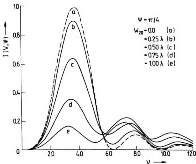
Fig. 2. Intensity point spread function of defocused polarizing microscope:  $\Psi = \pi/4$ ;  $W_{20} = 0.0, 0.25\lambda, 0.50\lambda, 0.75\lambda$  and  $1.0\lambda$
