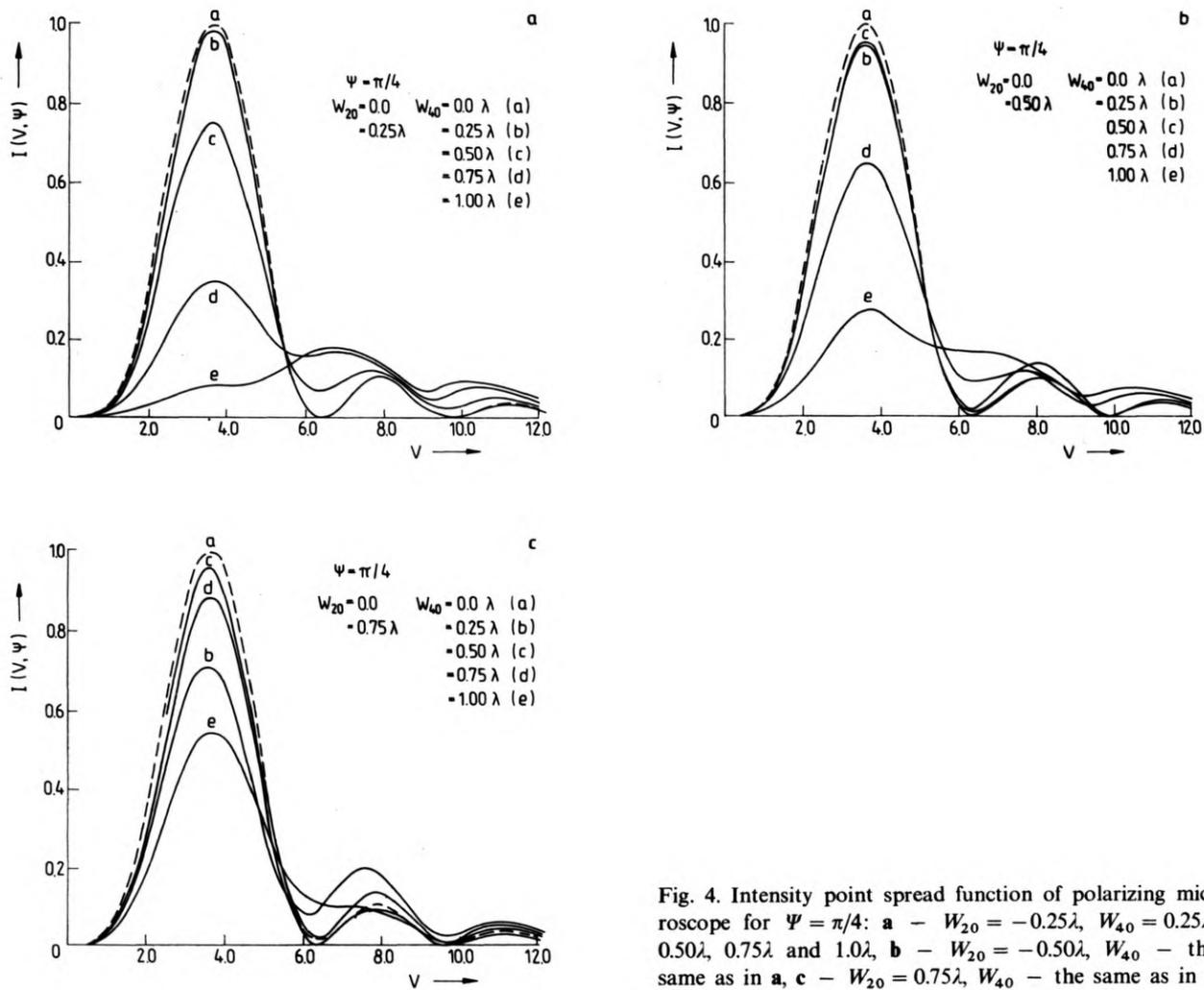
Fig. 4. Intensity point spread function of polarizing microscope for  $\Psi = \pi/4$ : **a** -  $W_{20} = -0.25\lambda$ ,  $W_{40} = 0.25\lambda$ ,  $0.50\lambda$ ,  $0.75\lambda$  and  $1.0\lambda$ , **b** -  $W_{20} = -0.50\lambda$ ,  $W_{40}$  - the same as in **a**, **c** -  $W_{20} = 0.75\lambda$ ,  $W_{40}$  - the same as in **a**
