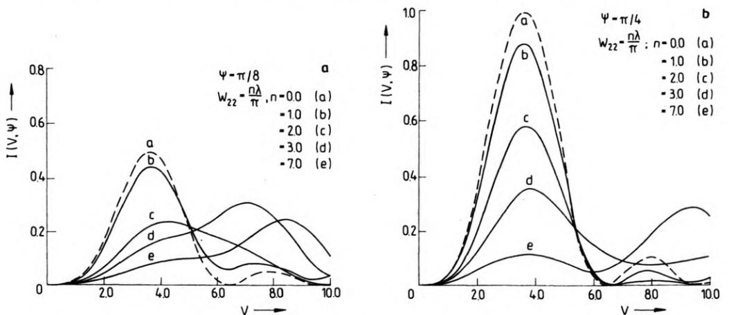
Fig. 6. Intensity point spread function in the presence of primary astigmatism: **a** -  $\Psi = \pi/8$ ,  $W_{22} = n\lambda/\pi$ ,  $n = 0.0, 1, 2, 3$  and  $7$ , **b** -  $\Psi = \pi/4$ ,  $W_{22}$  - the same as in **a**
