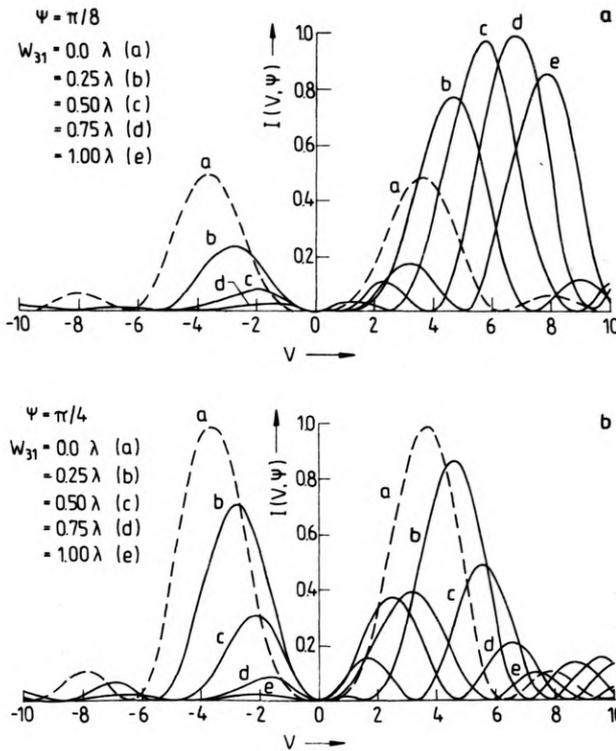
Fig. 5. Intensity point spread function of polarizing microscope in the presence of primary coma: **a** -  $\Psi = \pi/8$ ,  $W_{31} = 0.0, 0.25\lambda, 0.50\lambda, 0.75\lambda$  and  $1.0\lambda$ , **b** -  $\Psi = \pi/4$ ,  $W_{31}$  - the same as in **a**
