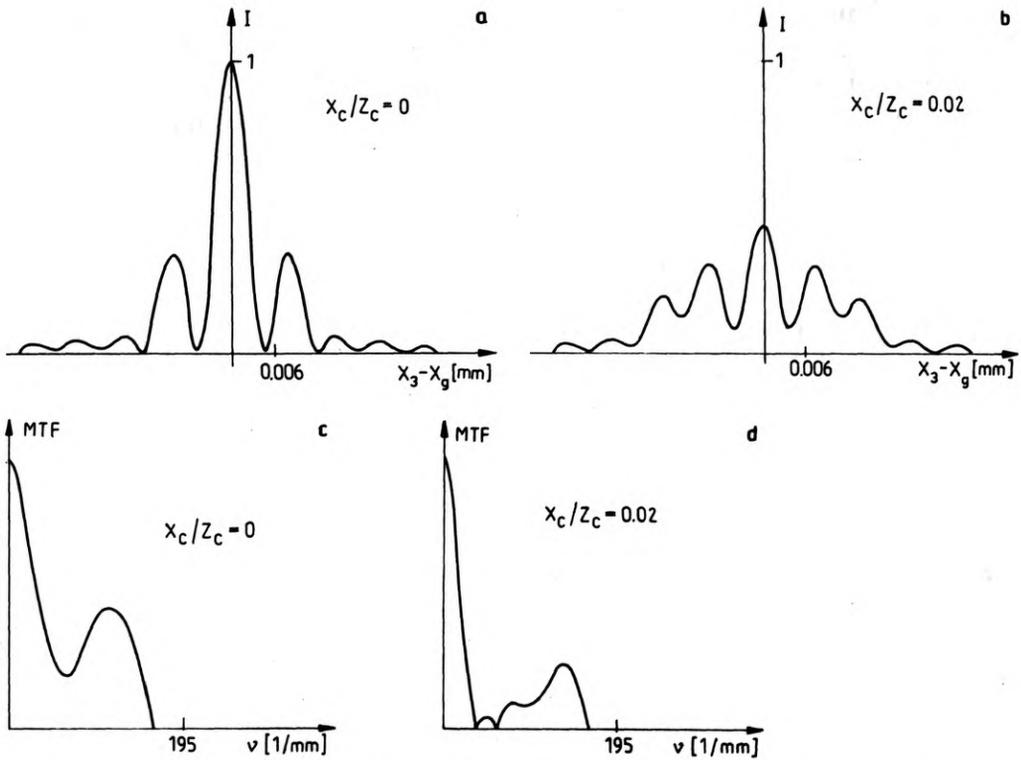
Fig. 1. Light intensity distribution ( $I$ ) in the aberration spot and incoherent modulation transfer function (MTF). For example No. 1
