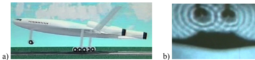
Fig.8 a) Artist impression of the 'silent plane' during landing; b) Simulation of the reduction of sound propagation from the engines mounted on the top of the plane. Pictures courtesy of Cambridge MIT Institute [17]
