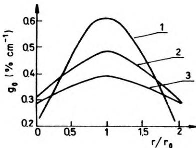
Fig. 1. Gaussian small signal gain variations along the gas flow directions [3] obtained by fitting experimental data corresponding to partial pressures  $p(\text{CO}_2)/p(\text{N}_2)$  equal to 1/2 (curve 1), 1/4 (curve 2), and 1/8 (curve 3), respectively, with a maximum on the resonator axis
