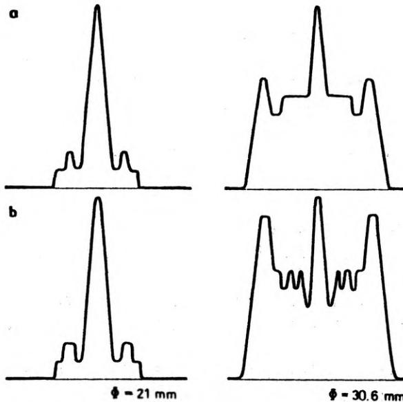
Fig. 4. Normalized near-field laser intensity distributions for small signal gain for curve 1 (a) and 3 (b) of Fig. 1 at two values of diaphragm diameter  $\phi$ . The central intensity on the resonator axis is used for normalization
