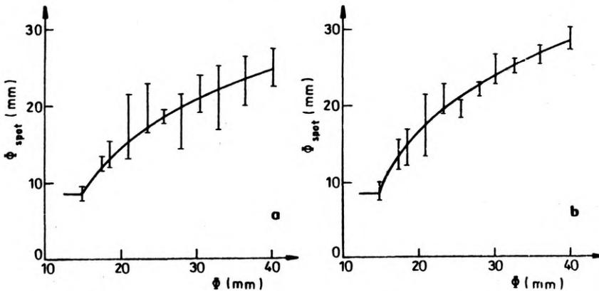
Fig. 5. Near-field laser spot diameter vs diameter of diaphragm adjacent to totally reflecting end mirror for small signal gain, curve 1 (a) and curve 3 (b)
