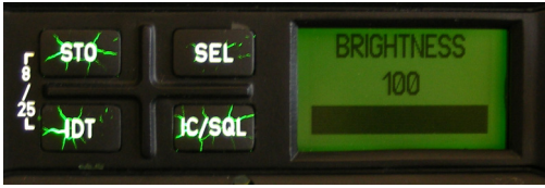
Fig. 1. First front panel version – lighting leakages.
