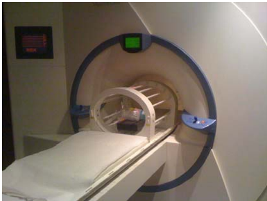
Fig. 8. Sonata scanner at the John Paul II Hospital with ^3\text{He} coil from RAPID Biomedical. In the center of the coil, a first phantom (see text) is placed for angle calibration experiment.
