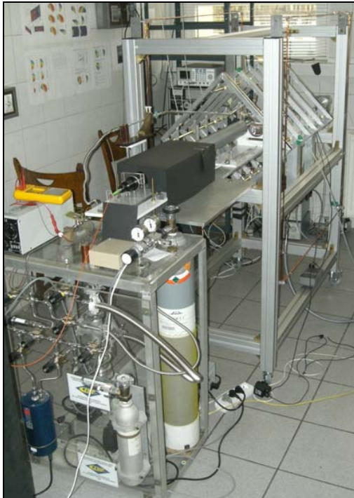
Fig. 1. Scheme of the table-top polarizer (see text). Six coils (cross-section) produce a homogeneous magnetic field. A gas handling system located under a 12 mm aluminium plate (G: getter, F: 50 \mu\text{m} filter) deliver gas to the optical pumping cell where it is being polarized by a laser tuned at 1083 nm (BS: polarizing beam splitter). The gas is then compressed to a storage cell (V: one-way valve, PI: pressure sensor) with a peristaltic compressor. The same gas can be compressed a second time to atmospheric pressure inside a syringe for rat lung experiment using a bypass between the input and output of the compressor.
