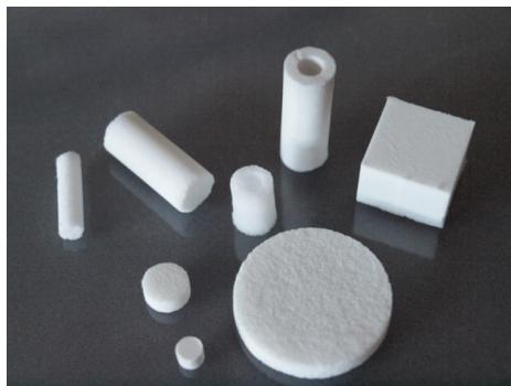
Fig. 4. The sintering process provides an alternative method to obtain monoliths with flexible geometric shape: tubes, rods, plates and granules could be prepared successfully.
