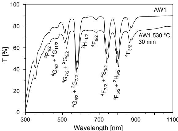
Fig. 3. Spectra transmittance of oxyfluoride AW1 parent glass and the glass after the heat treatment at 563 °C for 30 min.
