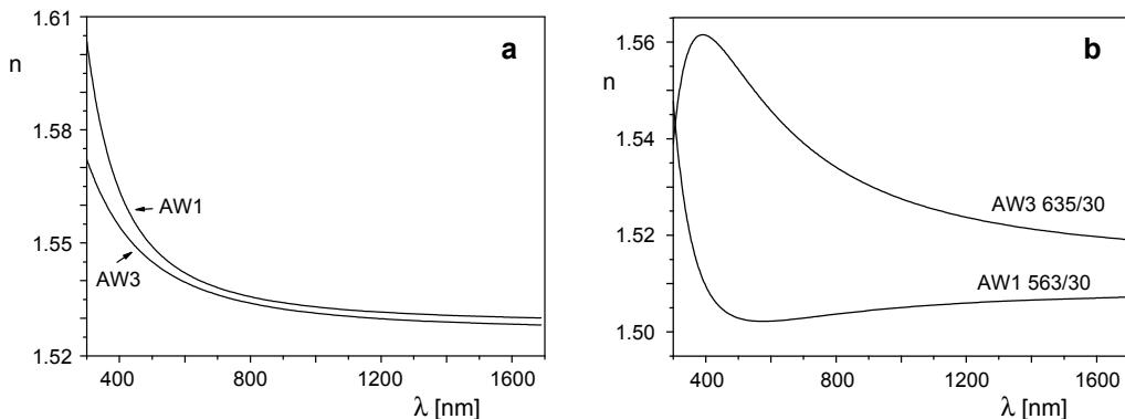
Fig. 6. Dispersion of  $n(\lambda)$  of glass (a) and oxyfluoride glass ceramic (b).
