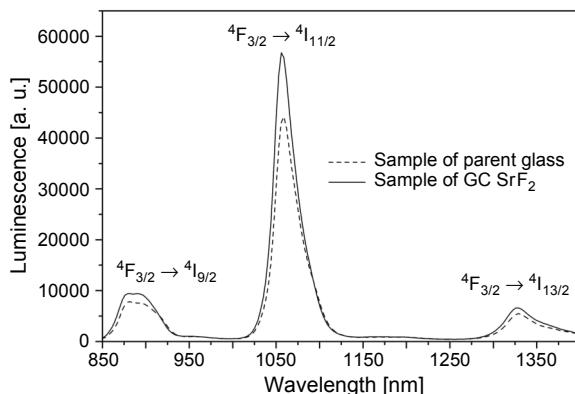
Fig. 7. Luminescence spectra of glass AW3 doped with Nd<sup>3+</sup> ions.
