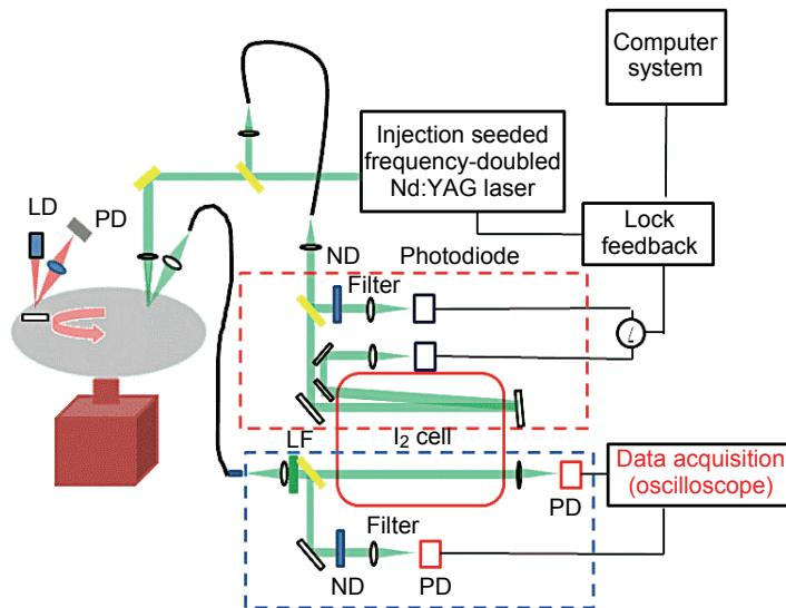
Fig. 3. Schematic diagram of the transmitting and receiving systems. A single iodine filter is used to lock the transmitter laser frequency and detect the Doppler frequency shift.
