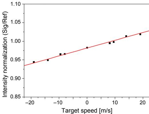
Fig. 7. Plot of changes in the transmitted signal against the actual speed of the rotating disc.
