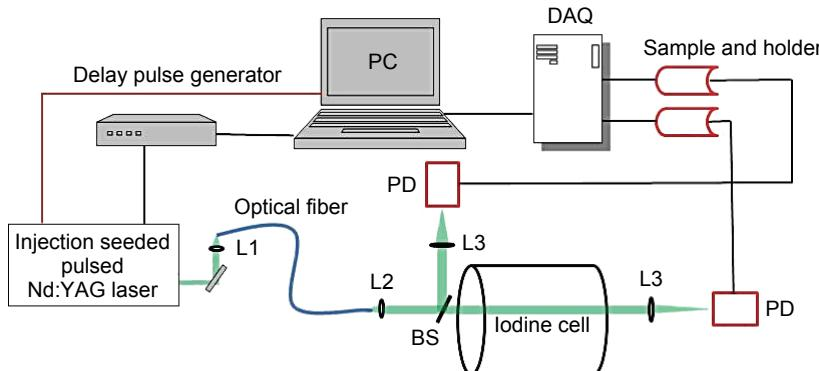
Fig. 4. Schematic diagram of laser frequency locking.
