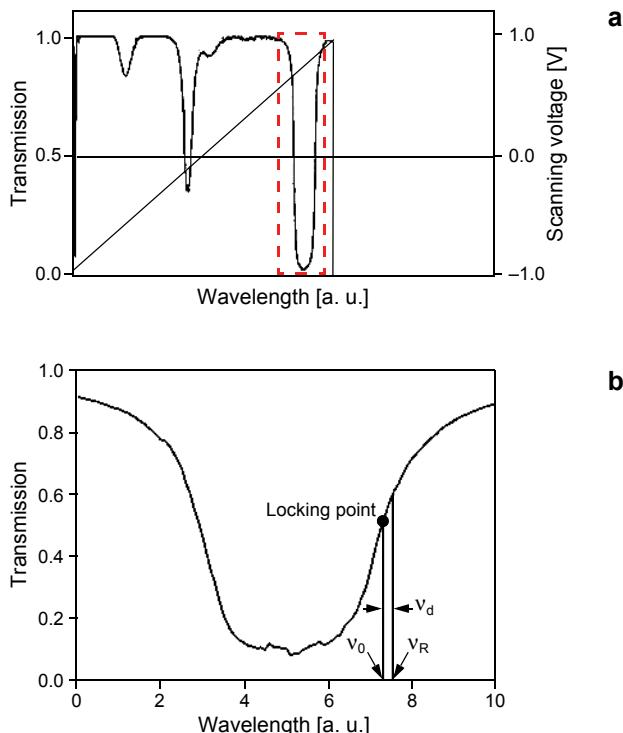
Fig. 1. Plots of iodine transmission ratio against tunable seeder laser wavelength for external input voltage of  $-1\text{ V}$  to  $+1\text{ V}$ , which is varied in steps of  $100\text{ }\mu\text{V}$  (a). Laser output at  $532\text{ nm}$  is locked to the halfway point on the edge of the iodine spectral absorption line (b).
