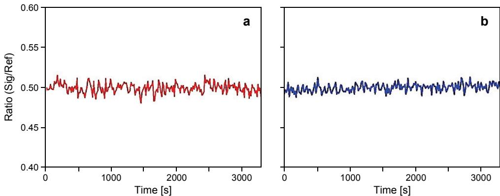
Fig. 5. Stability of laser frequency locking for iodine absorption line (a) and Fabry–Pérot etalon (b).
