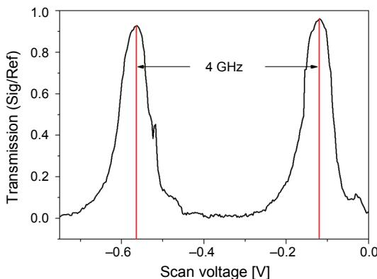
Fig. 2. Transmission ratio of Fabry–Pérot etalon with known free spectral range (FSR) of  $4 \text{ GHz}$ . This transmission ratio is measured by varying the frequency control input voltage from  $-1$  V to  $+1$  V in steps of  $100 \mu\text{V}$ .
