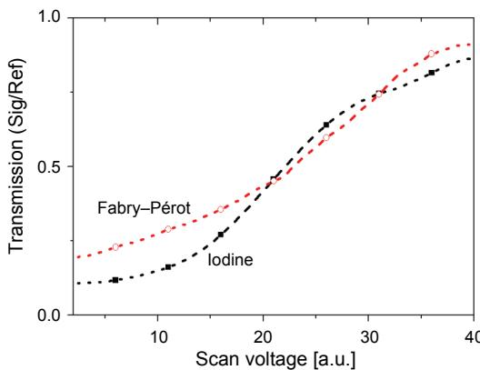
Fig. 6. Transmission ratios of iodine absorption and Fabry–Pérot etalon. The curve for iodine shows a steeper slope than that for the Fabry–Pérot etalon.
