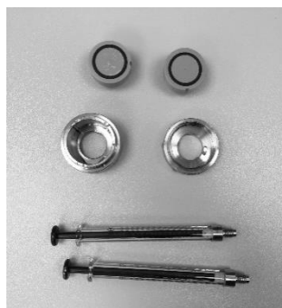
Fig. 2. The set of removable part in the extruder
