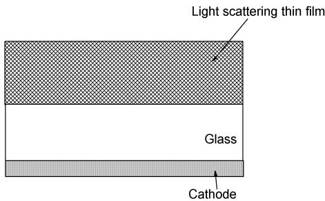
Fig. 1. The cross-section of a modeling device.
