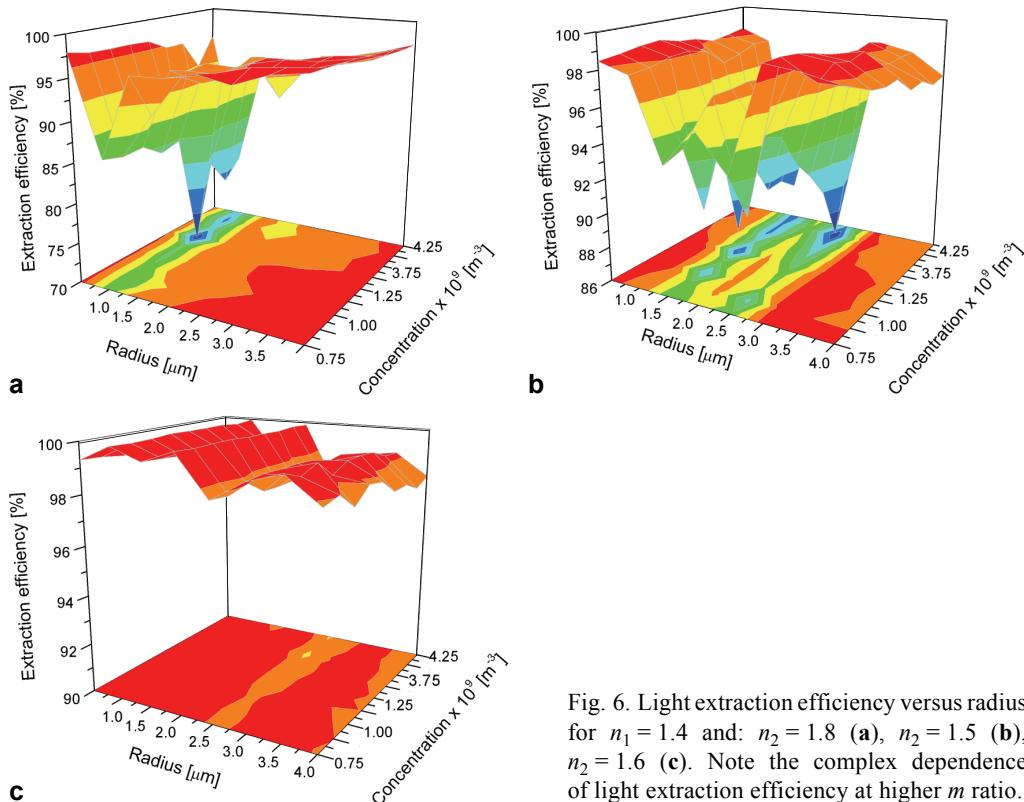
Fig. 6. Light extraction efficiency versus radius for  $n_1 = 1.4$  and:  $n_2 = 1.8$  (a),  $n_2 = 1.5$  (b),  $n_2 = 1.6$  (c). Note the complex dependence of light extraction efficiency at higher  $m$  ratio.
