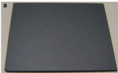
Fig. 15. SPS TiO 2 cathode with 50×50 mm 2 surface area (a) and the light source prototype model with such cathode (b).
