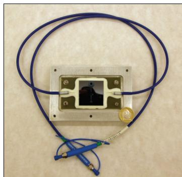
Fig. 2. Assembled LOC.
