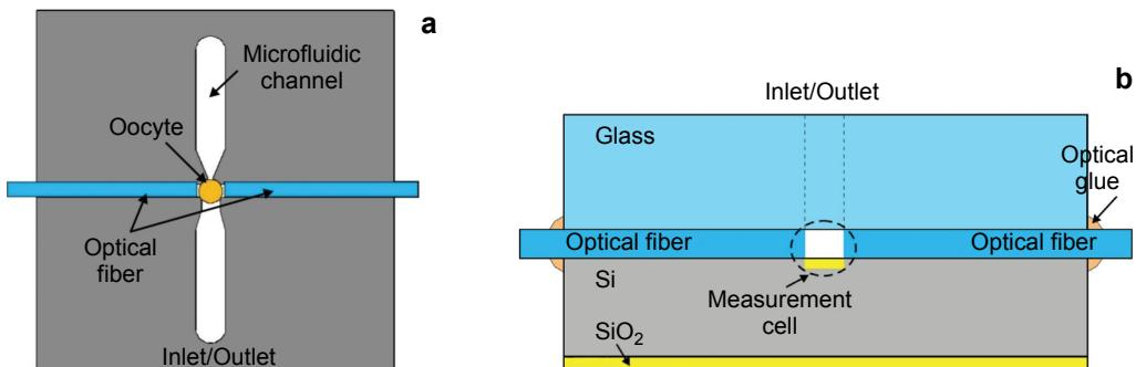
Fig. 1. Scheme (a) and cross-section (b) of the chip for characterization of living oocytes.
