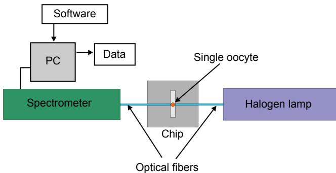
Fig. 4. Measurement set-up for pig oocytes microspectrometric characterization.
