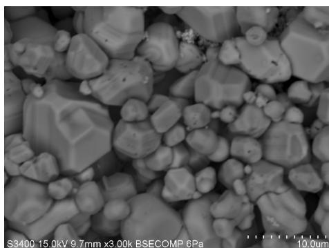
Fig. 2. SEM picture of ZnS:Cu powder, used in fabrication of EL thick-film structures.
