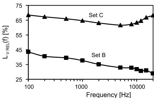
Fig. 4. Luminance of sets B and C of samples, relative to the luminance of set A, as a function of frequency, for a 100 V square-wave excitation.
