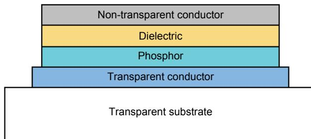
Fig. 1. Cross-section of a thick film electroluminescent lamp.
