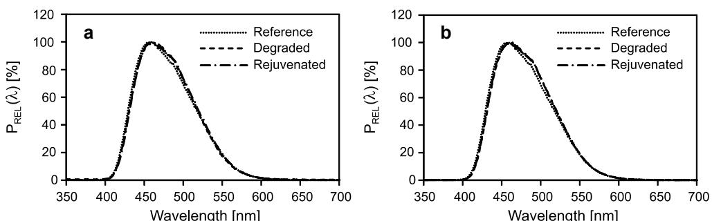
Fig. 8. Normalized spectrum of light emission of set B (a) and set C (b) samples, for a 100 V, 2 kHz square-wave excitation.
