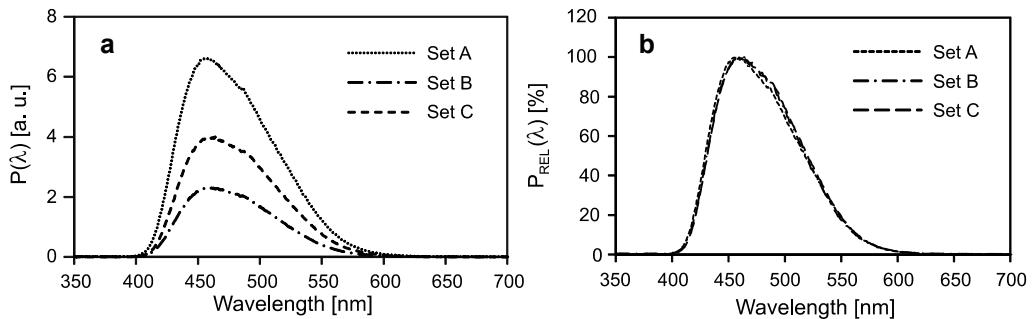
Fig. 5. Spectrum of light emission (a) and normalized spectrum of light emission (b), for a 100 V, 2 kHz square-wave excitation.
