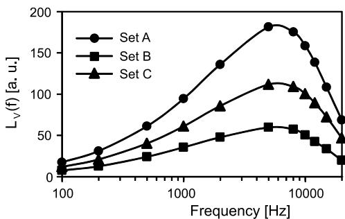
Fig. 3. Luminance as a function of frequency for samples from sets A, B and C, for a 100 V square-wave excitation.
