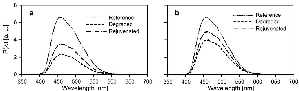
Fig. 7. Spectrum of light emission of set B (a) and set C (b) samples, for a 100 V, 2 kHz square-wave excitation.
