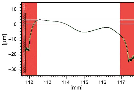
Fig. 6. Profilometry measurement of glaze strip printed on sol-gel films.
