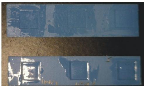
Fig. 4. Sample with glaze in cavities on DP951 substrates after firing.
