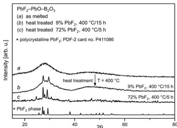
Fig. 1. X-ray diffraction patterns for oxyfluoride lead borate glasses before and after thermal treatment.
