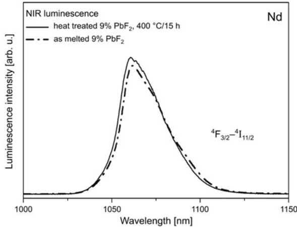
Fig. 2. Luminescence spectra at 1.06  $\mu\text{m}$  recorded for  $\text{Nd}^{3+}$  ions in glass samples before and after thermal treatment. NIR luminescence bands correspond to the main  ${}^4F_{3/2}-{}^4I_{11/2}$  laser transition of  $\text{Nd}^{3+}$  ions.
