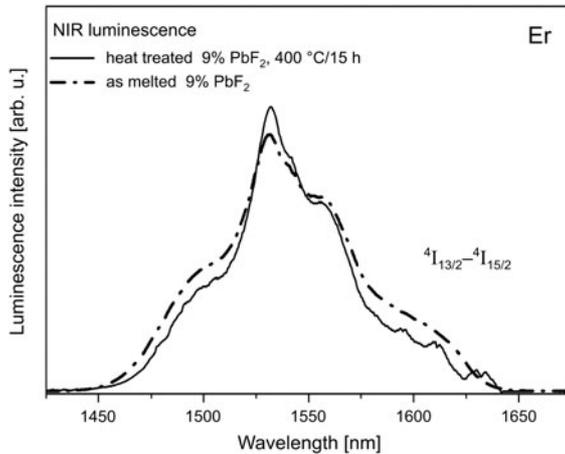
Fig. 3. Luminescence spectra at 1.53  $\mu\text{m}$  recorded for  $\text{Er}^{3+}$  ions in glass samples before and after thermal treatment. NIR luminescence bands correspond to the main  ${}^4I_{13/2}-{}^4I_{15/2}$  laser transition of  $\text{Er}^{3+}$  ions.
