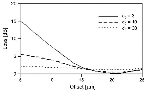
Fig. 4. Modal filtering loss for the data from Fig. 3 for various coupling coefficients  $d(x) = d_0$  [1/km].
