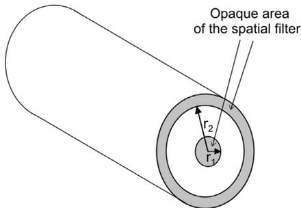
Fig. 6. View of the fiber core end surface. A spatial filter that realizes the transfer function in Fig. 5 is applied. The fiber cladding is not shown.
