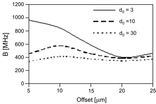
Fig. 2. Modal bandwidth in the presence of modal filtering with the filter (16) and for a distorted profile (15), launch beam diameter is  $9 \mu\text{m}$ ,  $d(x) = d_0 = \text{const}$  [1/km].
