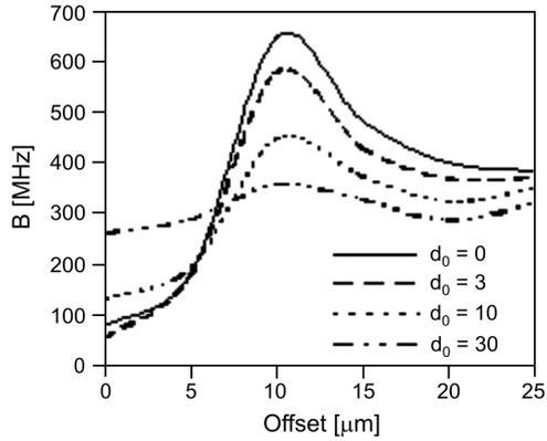
Fig. 1. Modal bandwidth  $B$ , versus offset: the exciting beam diameter is  $9 \mu\text{m}$ ,  $d(x) = d_0 = \text{const}$  [1/km]. The profile is distorted according to (15):  $h = 0.5$  and  $x_0 = 0.05$ .
