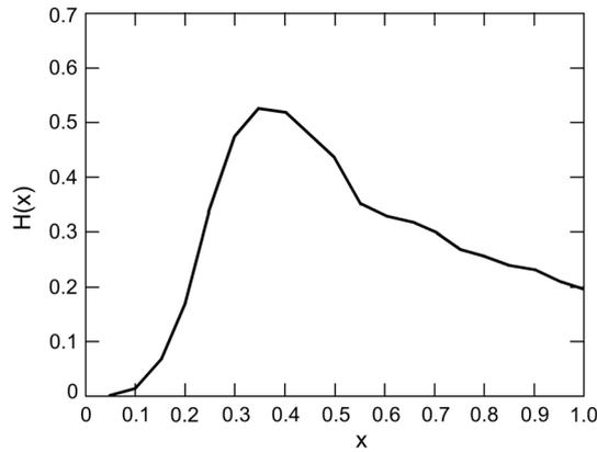
Fig. 5. Transfer function  $H(x)$  realized in a MM fiber ( $\lambda = 0.78 \mu\text{m}$ ,  $D = 50 \mu\text{m}$ ,  $g = 2$ ,  $\text{NA} = 0.2$ ,  $n_1 = 1.48$ ) by a circular diaphragm located at the fiber end that is opaque for  $r < 10 \mu\text{m}$  and for  $r > 15 \mu\text{m}$ , and transparent elsewhere.
