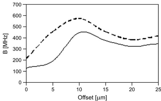
Fig. 3. Modal bandwidth in the absence of modal filtering (solid line), and in its presence (dashed line). Modal filtering is with the filter (16) and for the distorted profile (15), launch beam diameter is  $9 \mu\text{m}$ ,  $d(x) = d_0 = 10$  [1/km]. Modal filtering loss does not exceed here 6.1 dB.
