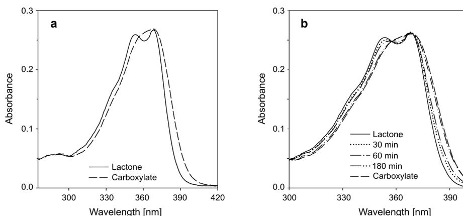
Fig. 4. Absorption spectra of lactone and carboxylate forms of camptothecin recorded in PBS at pH 7.4 (a). The series of absorption spectra of camptothecin recorded during the hydrolysis process in PBS at pH 7.4 (b). The first one is the lactone form spectrum (solid line), the subsequent spectra were recorded 30, 60 and 180 minutes after sample preparation. The last one is the spectrum of the carboxylate form (dashed line).
