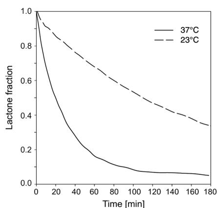
Fig. 5. Time dependence of the fraction of the lactone form obtained from factor analysis of a series of absorption spectra recorded during the hydrolysis process of camptothecin in PBS at pH 7.4 and temperatures of 23 and 37°C.
