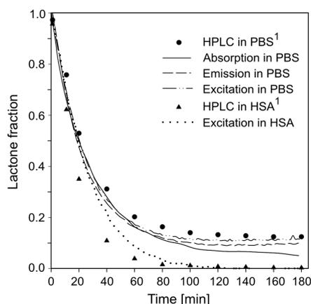
Fig. 8. Comparison of the results of the rate of camptothecin hydrolysis obtained from factor analysis of emission, excitation and absorption spectra and the HPLC method. The measurements were performed in PBS and HSA at pH 7.4 and a temperature of 37°C (<sup>1</sup>Previously reported results [4, 5] obtained from HPLC measurements).
