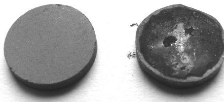
Fig. 8. BIMEVOX before (left) and after measurement in reducing atmosphere (right)
