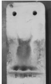
Fig. 8. The methacrylate CP specimen after testing for resistance to tracking at 6 kV
