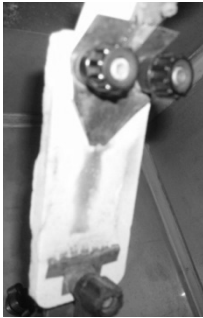
Fig. 7. Electrodised specimen during testing for resistance to tracking currents
