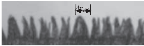
Figure 10. Graphical definition of \Delta x_{chip}
