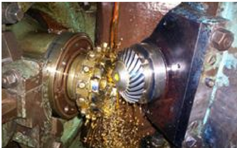
Fig. 26.6. A Gleason face mill cutter in operation [The Gleason Works]
