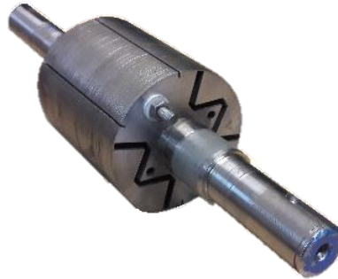
Fig. 2.14. Isometric view of the built rotor without magnets
