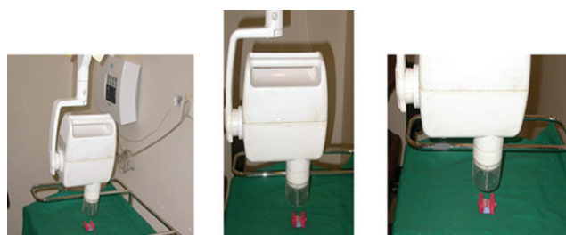
Fig. 4. Adjusting the X-ray tube angulation to take radiographs at different horizontal angles
