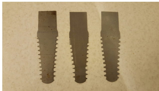
Fig. 3. Three models of dental implants with different thread designs
