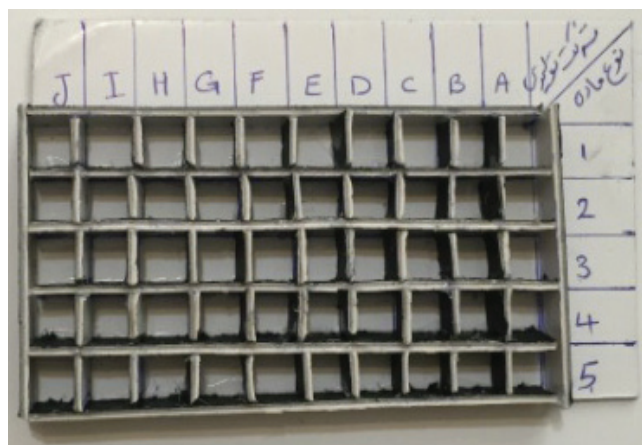
Fig. 1. A cardboard grid fabricated for the placement of the restorative materials
