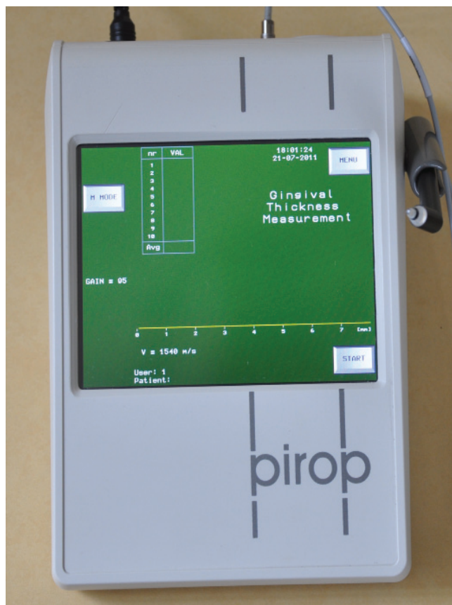
Fig. 1. PIROP® (Echo-Son S.A., Puławy, Poland) Specifications: probe frequency – 20 MHz; velocity range – 1400–3000 m/s; measurement range – 0.25–6 mm; axial resolution – 0.01 mm (10 \mu m); 4 predefined maps of periodontal areas.
