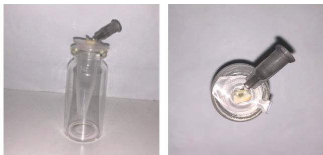
Fig. 1. Experimental system used to evaluate the debris extrusion
