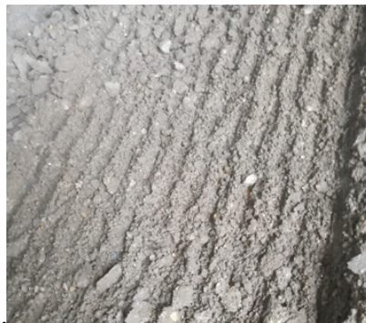
Fig. 10. The fracture zone formed on the surface of the coal-rock
