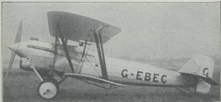
Vickers „Vixen VI“ (1927) Ka 2; E: R. Pierson b = 13,74 m; l = 10,51 m; T = 54,81 m 2 ; L = 1,72 t; N = 0,79 t; G = 2,51 t; V = 82–238 km/h; H = 8,6 km; St = 4,5 km/13'; M: Rolls Royce 700 PS-HP-CV; Bst.: H, St.
