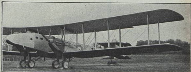
Armstrong Whitworth „Awana“ (1923) Ktr; E: F. M. Green b = 32,20 m; l = 20,70 m; T = 214,0 m 2 ; L = 4,53 t; N = 3,22 t; G = 7,75 t; V = 156 km/h; H = 3,4 km; M: 2 × Napier 450 PS-HP-CV = 900 PS-HP-CV; Bst.: H, St. S.
