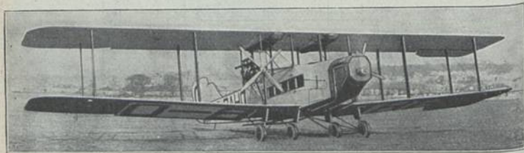
Handley Page W 8 F (1924) V 12; E: F. Handley Page b = 22,86 m; l = 18,31 m; T = 136,1 m 2 ; L = 3,89 t; N = 1,99 t; G = 5,88 t; V = 83–164 km/h; H = 3,1 km; St = 0,51 km/1'; M: 1 × Rolls Royce 360 PS-HP-CV, 2 × Siddeley 240 PS-HP-CV = 840 PS-HP-CV; Bst.: H. St.
