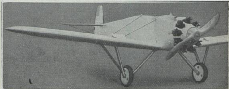
Koolhoven F K 35 (1926) Kj 2; E: F. Koolhoven b = 11,50 m; l = 8,60 m; T = 24,00 m 2 ; L = 0,90 t; N = 0,64 t; G = 1,54 t; V = 85–260 km/h; H = 7,8 km; St = 5,0 km/14'; M: Bristol 450 PS-HP-CV; Bst.: H. S. St.
