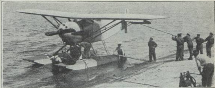
Koolhoven F K 34 (1926) Kaw 2; E: F. Koolhoven b = 13,00 m; l = 9,30 m; L = 1,70 t; N = 0,80 t; G = 2,50 t; V = 204 km/h; M: Hispano 450 PS-HP-CV; Bst.: H. St.
