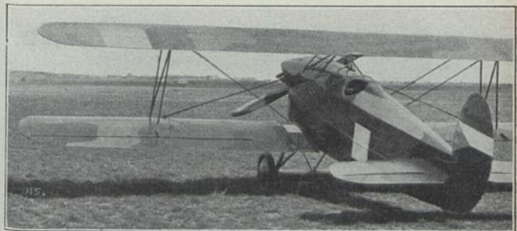
Avia B H 22 (1925) U 1; E: Benes, Hajn b = 8,90 m; l = 6,66 m; T = 22,00 m 2 ; L = 0,68 t; N = 0,18 t; G = 0,86 t; V = 85—216 km/h; H = 6,5 km; St = 5,0 km/20'; M: Hispano 180 PS-HP-CV; Bst.: H, St, S.
