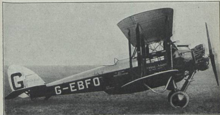
de Havilland D. H. 50 J (1926) V 4; E: G. de Havilland b = 13,30 m; l = 9,30 m; T = 67,00 m 2 ; G = 1,77 t; M: Siddeley 385 PS-HP-CV; Bst.: H, St. The de Havilland Aircraft Co. Ltd., Stag Lane, Edgware, Middlesex
