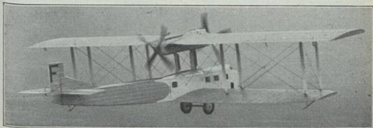
Farman F 180 „Oiseau-bleu“ (1927) V 27; E: Farman b = 26,00 m; l = 13,00 m; T = 175,0 m 2 ; L = 4,50 t; N = 3,30 t; G = 7,80 t; V = 190 km/h; H = 4,0 km; M: 2 × Farman 500 PS-HP-CV = 1000 PS-HP-CV; Bst.: H. St.
