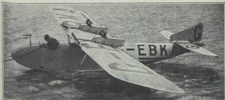
Short „Stellite“ (1924) Sps 2; E: M. Short b = 10,97 m; l = 7,52 m; T = 19,00 m 2 ; L = 0,37 t; N = 0,10 t; G = 0,40 t; V = 61–110 km/h; M: 2 × Blackburne 18 PS-HP-CV = 36 PS-HP-CV; Bst.: S, St, D.
