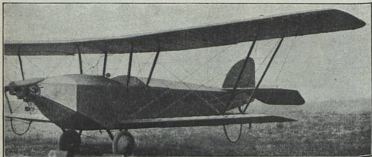
Cranwell C. L. A. 2. (1924) Sp 2; E: Comper b = 9,05 m; l = 7,17 m; T = 17,10 m 2 ; L = 0,23 t; N = 0,17 t; G = 0,40 t; V = 48–89 km/h; M: Bristol 36 PS-HP-CV; Bst.: H, St.
