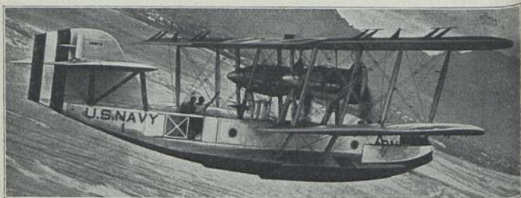
U. S. Navy P N 9 (1924) Ks 3; E: G. C. Westervelt b = 22,50 m; l = 15,00 m; T = 125,0 m 2 ; L = 4,07 t; N = 0,72 t; G = 4,89 t; M: 2 × Packard 480 PS-HP-CV = 960 PS-HP-CV; Bst.: H, S, St.
