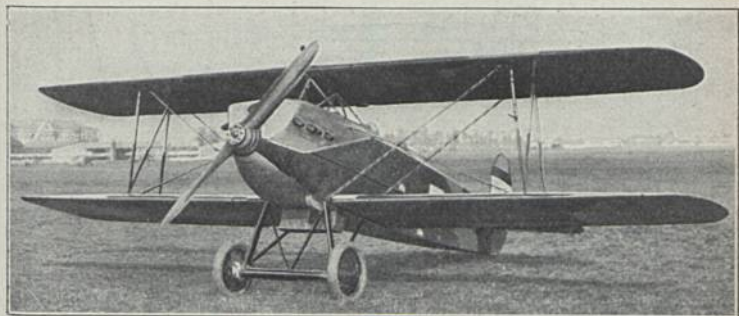
Avia B H 21 s (1925) K1 1; E: Benes, Hajn b = 8,90 m; l = 6,87 m; T = 22,00 m 2 ; L = 0,76 t; N = 0,32 t; G = 1,08 t; V = 90—246 km/h; H = 8,0 km; St = 5,0 km/13'; M: Hispano 300 PS-HP-CV; Bst.: H, St.
