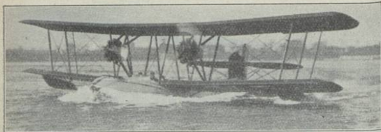
Canadian Vickers „Varuna“ (1925) Ksa 4; E: W. T. Reid b = 16,84 \text{ m} ; l = 11,66 \text{ m} ; T = 69,00 \text{ m}^2 ; L = 1,68 \text{ t} ; N = 0,90 \text{ t} ; G = 2,58 \text{ t} ; V = 71\text{--}145 \text{ km/h} ; M: 2 \times \text{Wright } 200 \text{ PS-HP-CV} = 400 \text{ PS-HP-CV} ; Bst.: H. St.
