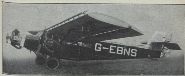
Handley Page „Hamlet“ (1926) V 5; E: F. Handley Page b = 15,80 m; l = 10,59 m; T = 36,08 m 2 ; L = 1,66 t; N = 0,69 t; G = 2,35 t; V = 72–188 km/h; H = 3,2 km; St = 0,19 km/1'; M: 3 × Bristol 120 PS-HP-CV = 360 PS-HP-CV; Bst.: H, St, S.
