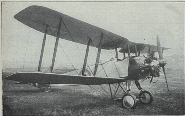
Avro 504 N (1924) Ü 2; E: A. V. Roe b = 10,97 m; l = 8,83 m; T = 29,70 m 2 ; L = 0,71 t; N = 0,27 t; G = 0,98 t; V = 66–153 km/h; H = 5,4 km; M: Siddeley 180 PS-HP-CV;
