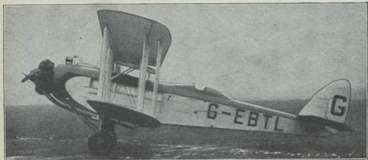
de Havilland D. H. 61 „Canberra“ (1928) V 9; E: G. de Havilland b = 16,95 m; l = 14,00 m; T = 57,00 m 2 ; L = 1,42 t; N = 0,86 t; G = 2,28 t; V = 76–203 km/h; H = 4,5 km; M: Bristol 450 PS-HP-CV; Bst.: H, St.
