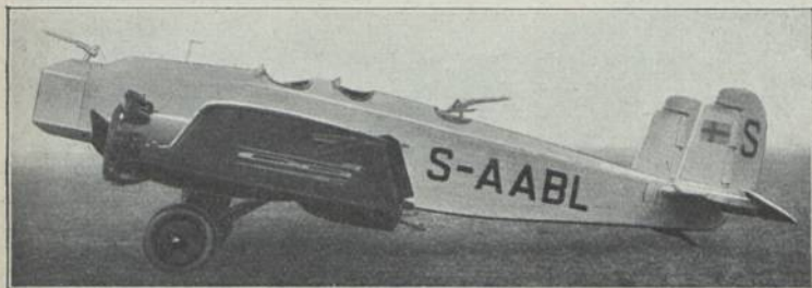
Junkers K 37 L (1927) Kb 5; E: Junkers b = 20,00 m; l = 11,35 m; T = 47,20 m 2 ; L = 2,30 t; N = 1,30 t; G = 3,60 t; V = 224 km/h; H = 7,2 km; M: 2 × Gnôme 480 PS-HP-CV = 960 PS-HP-CV; Bst.: D.
