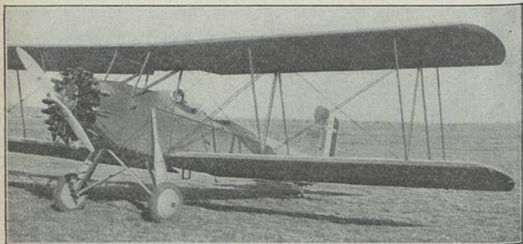
Curtiss X N 2 C-1 „Fleagling“ (1928) Ka 2; E: T. P. Wright b = 11,90 m; l = 8,20 m; T = 33,70 m 2 ; L = 0,90 t; N = 0,30 t; G = 1,20 t; V = 72–177 km/h; H = 3,0 km; M: Wright 200 PS-HP-CV; Bst.: H, S, St.
