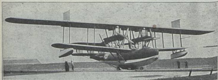
Fairey N 4 „Atalanta“ (1924) Ksb 4; E: C. R. Fairey b = 42,36 m; l = 20,11 m; T = 27,00 m 2 ; G = 13,6 t; M: 4 × Rolls Royce 600 PS-HP-CV = 2400 PS-HP-CV; Bst.: H, St.
