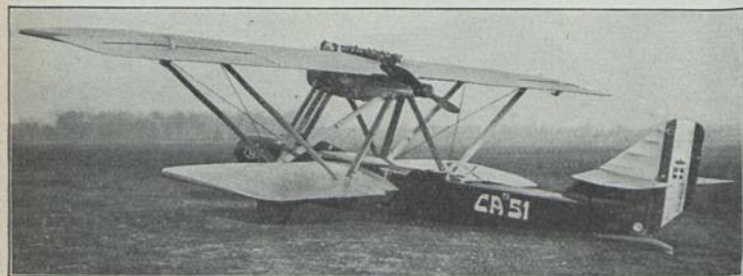
Caproni Ca 70 L (1926) K1 2; E: G. Caproni b = 17,00 m; l = 8,54 m; T = 55,00 m 2 ; L = 1,31 t; N = 0,82 t; G = 2,13 t; V = 90–200 km/h; St = 4,0 km/17'; M: Lorraine 400 PS-HP-CV; Bst.: H, St.
