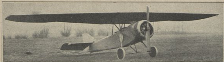
Junkers U 23 E (1924) U 2; E: Junkers b = 13,60 m; l = 7,50 m; M: Le Rhône 110 PS; 1 st.: Dural
