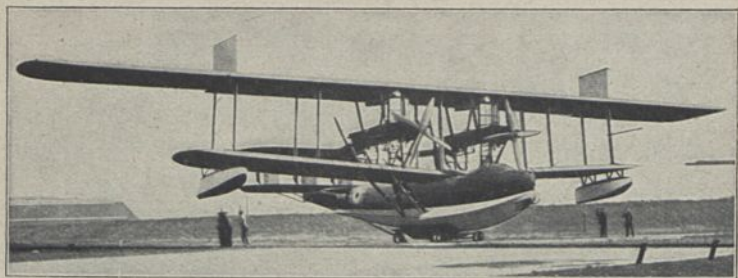
Fairey N 4 „Atlanta“ (1924) Ksb 4; E: C. R. Fairey b = 42,36 m; l = 20,11 m; T = 270,00 qm; G = 13,60 t; M: 4 \times Rolls Royce 600 PS = 2400 PS; MG: 4; Bst.: Holz, Stoff Fairey Aviation Co. Ltd., Hayes, Middlesex
