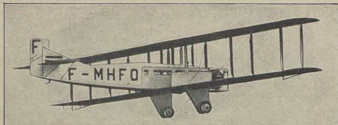
Farman F 60c „Goliath“ (1923) V 16; E: Farman b = 26,50 m; l = 14,77 m; T = 161,00 qm; L = 2,50 t; N = 2,50 t; G = 5,00 t; V = 160 km/h; M: 2 × Salmson 260 PS = 520 PS; Bst.: Holz, Stoff
