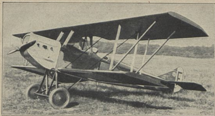
Morane-Saulnier 43 E T 2 (1924) U 2; E: R. Saulnier b = 10,82 m; l = 7,86 m; T = 28,05 qm; L = 0,80 t; N = 0,32 t; G = 1,12 t; V = 164 km/h; H = 5,5 km; M: Hispano 180 PS; Bst.: Dural, Stahl, Holz, Stoff
