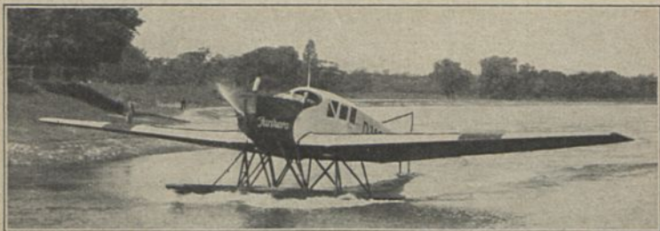
Junkers F 13 W (1921) V 6; E: Junkers b = 17,75 m; l = 10,15 m; T = 40,00 qm; L = 1,35 t; N = 0,60 t; G = 1,95 t; V = 170 km/h; M: BMW 185 PS; Bst.: Dural
