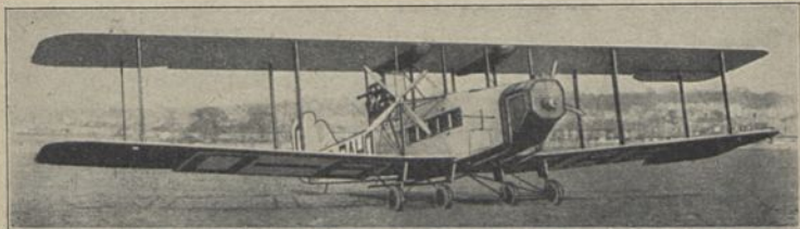
Handley Page W 8 F (1924) V 12; E: F. Handley Page b = 22,80 m; l = 18,30 m; T = 135,00 qm; L = 4,30 t; N = 1,16 t; G = 5,46 t; V = 164 km/h; M: 2 × Siddeley 240 PS; 1 × Rolls Royce 360 PS = 840 PS; Bst.: Holz, Stoff
