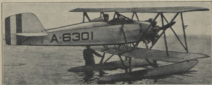
U. S. Navy TR 1 (1923) Kaw 1; E: J. C. Hunsaker b = 7,62 m; l = 7,50 m; T = 21,00 qm; G = 0,81 t; V = 210 km/h; M: Lawrance 220 PS; Bst.: Holz, Stahl, Stoff
