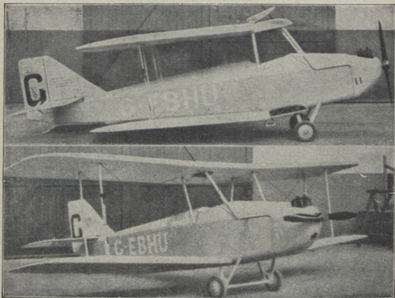
Gloucestershire „Gannet“ (1923) Sp 1; E: H. Folland b = 5,50 m; l = 5,10 m; T = 9,85 qm; L = 0,12 t; N = 0,08 t; G = 0,20 t; M = Carden 24 PS; Bst.: Holz, Stoff Gloucestershire Aircraft Co. Ltd., Cheltenham
