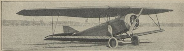
Junkers U 23 D (1924) U 2; E: Junkers b = 13,60 \text{ m} ; l = 7,50 \text{ m} ; T = 32,00 \text{ qm} ; N = 0,86 \text{ t} ; V = 140 \text{ km/h} ; M: Le Rhône 110 PS; Bst.: Dural
