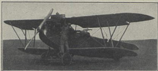
Phoenix C 1 (1918) Ka 2; E: L. Kirste b = 11,00 m; l = 7,80 m; T = 29,00 qm; L = 0,82 t; N = 0,42 t; G = 1,24 t; V = 170 km/h; H = 5,0 km; M: Hiero 230 PS; MG: 2; Bst.: Holz, Stoff
