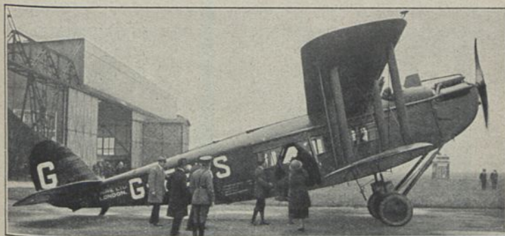
de Havilland D. H. 34. (1922) V 10; E: G. de Havilland b = 15,50 m; l = 11,18 m; L = 1,56 t; N = 1,29 t; G = 2,85 t; V = 150 km/h; M: Napier 450 PS; Bst: Holz, Stoff
