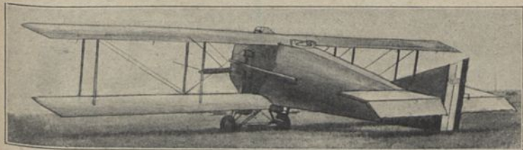
Farman B 2 (1923) Kb 2; E: Farman b = 17,00 m; l = 10,70 m; T = 63,00 qm; L = 1,36 t; N = 1,10 t; G = 2,46 t; V = 185 km/h; M: Lorraine 370 PS; MG: 4; Bst.: Dural
