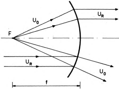
Fig. 3. Ray tracing of two unaberrated wave fronts through the curved Fourier transform holographic lens
