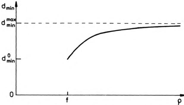
Fig. 2. Graphical representation of a functional relation between the minimal period of HOE and the curvature radius
