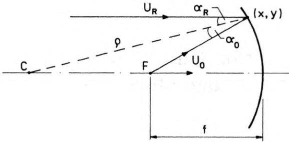
Fig. 1. Recording geometry of the HOE phase function on a spherical substrate
