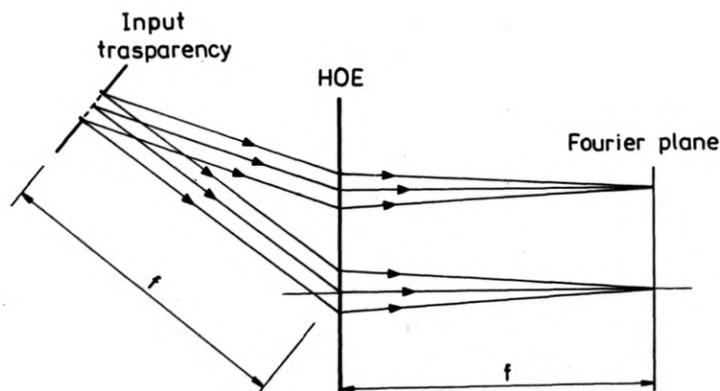
Fig. 5. Fourier transform off-axis HOE configuration
