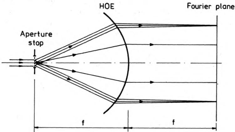
Fig. 4. Infinitesimal beams of diffracted rays at transparency focused in corresponding points of the output plane
