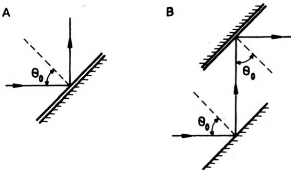
Fig. 1. One- and two-reflection thin-film phase retarding systems; the system A contains one thin-film coated mirror, and the two-reflection system B contains two mirrors, one coated and the other uncoated
