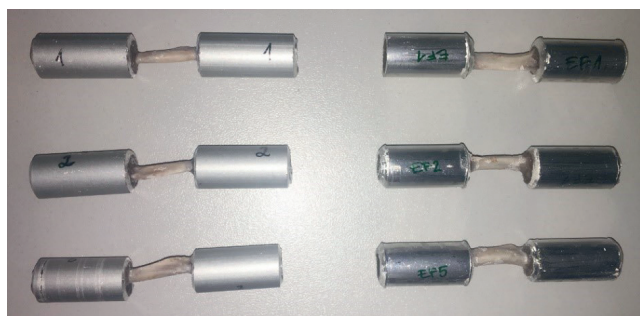
Fig. 1. Samples prepared for the four-point bending test
