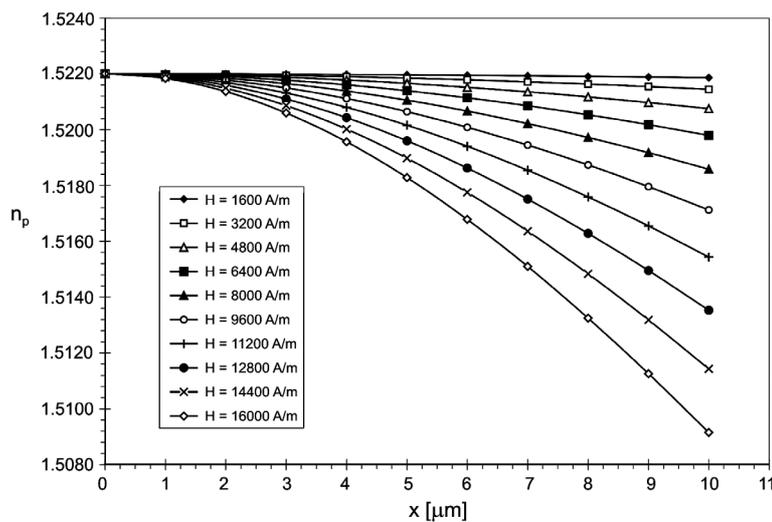
Fig. 4. Calculated refractive index profiles of FN layer for growing values of magnetic field intensity.
