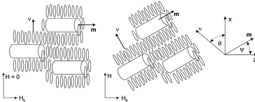
Fig. 2. Structure of ordered FN layer and its orientation change under influence of magnetic field ( $v$ – nematic liquid crystal director,  $\mathbf{m}$  – unit vector of ferroparticle magnetization director,  $\theta$ – nematic molecule tilt angle,  $\psi$ – ferroparticle magnetic moment tilt angle).
