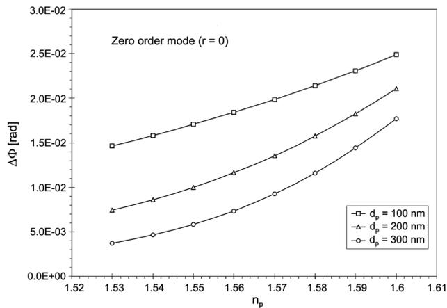
Fig. 5. Phase change of a zero order TM mode in magnetic field of intensity  $H = 16000$  A/m vs. refractive index of ordering layer  $n_p$  for different values of ordering layer thickness  $d_p$ .
