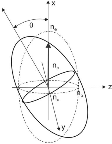
Fig. 3. Change of a spatial structure of the ferronematic layer's refractive index ellipsoid ( $n_c$  – refractive index of FN layer for TM mode).
