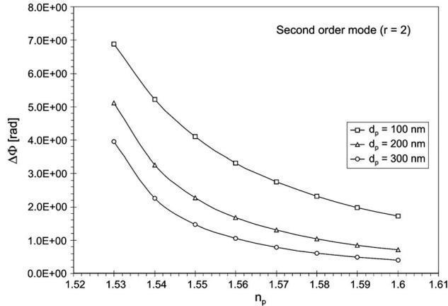
Fig. 7. Phase change of a second order TM mode in magnetic field of intensity  $H = 16000$  A/m vs. refractive index of ordering layer  $n_p$  for different values of ordering layer thickness  $d_p$ .
