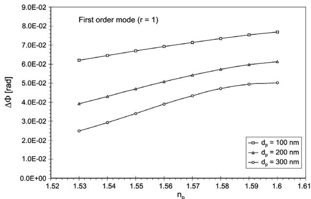
Fig. 6. Phase change of a first order TM mode in magnetic field of intensity  $H = 16000$  A/m vs. refractive index of ordering layer  $n_p$  for different values of ordering layer thickness  $d_p$ .
