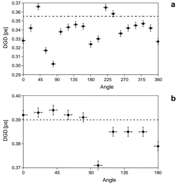
Fig. 7. DGD as a function of force direction for: **a** – *BlazePhotonics* PM 1550 01 and **b** – HB bow-tie fiber (dashed line represents the average value of non-stressed HB fiber).
