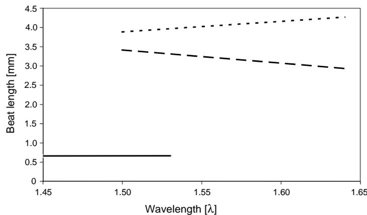
Fig. 3. Beat length as a function of wavelength for: HB PCF (UMCS) (solid line), *BlazePhotonics* PM 1550 01 (dashed line) and HB bow-tie (dotted line) fibers.
