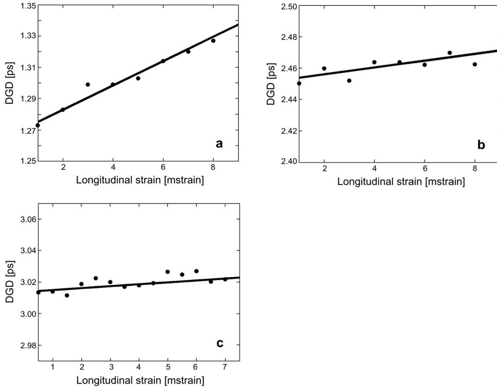
Fig. 5. DGD dependence on longitudinal strain for: bow-tie – **a**, HB PCF (UMCS) – **b**, *BlazePhotonics* PM 1550-01 – **c**.
