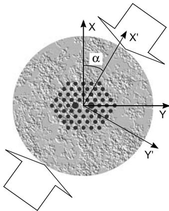
Fig. 6. Influence of axial stress that depends on the angle between birefringence axes and force direction.
