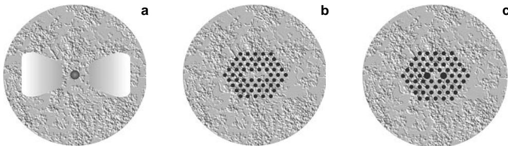
Fig. 1. Types of the HB fibers under investigation: *Fibercore* bow-tie – a, HB PCF (UMCS) – b, *BlazePhotonics* HB 1550 01 – c.
