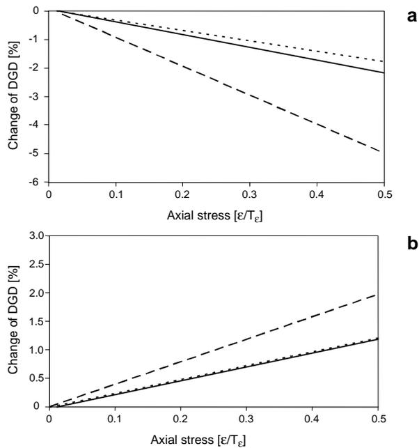
Fig. 8. Total change of DGD as a function of external stress for: **a** – 45 and **b** – 135 degrees between force direction and birefringence axes in the bow tie (dotted line), HB PCF (UMCS) (dashed line) and *BlazePhotonics* PM 1550 01 (solid line) HB fibers.
