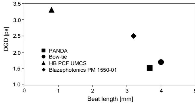
Fig. 4. Dependence of DGD on beat length for different types of HB fibers.
