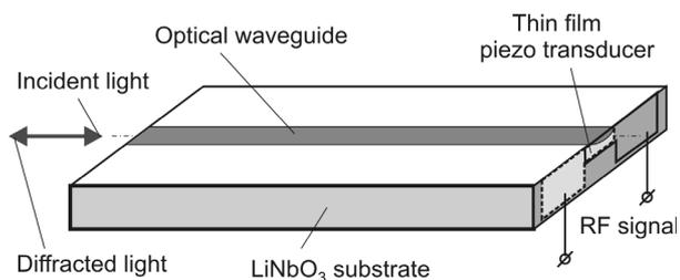
Fig. 7. Integrated collinear AO tunable mirror.
