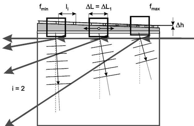
Fig. 4. Moving window multielement transducer system for Bragg angle and resonant frequency automatic tuning.
